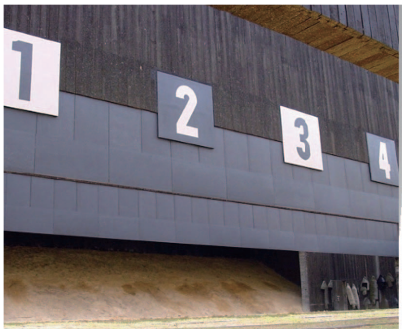
Bullet containment and catcher system at an outdoor live-firing range
