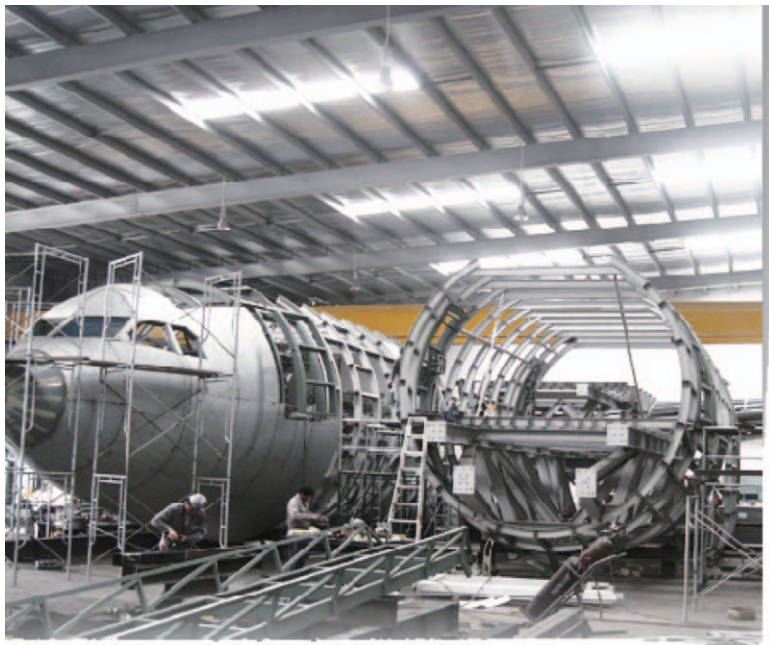
Fabrication of an aircraft mock-up
